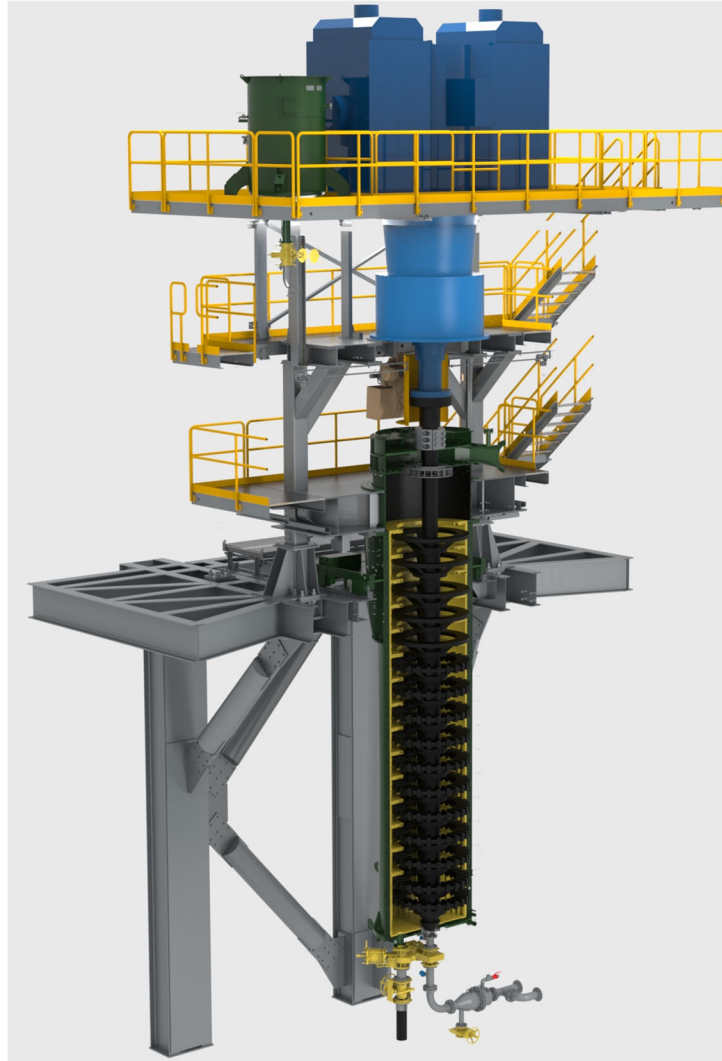
Figure 1—Typical VRM mill cross section
