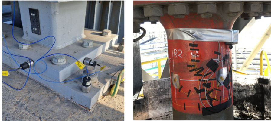
Figure 9—Left: Vibration sensors on the mill frame feet; Right: strain gauge set-up on the mill shaft
