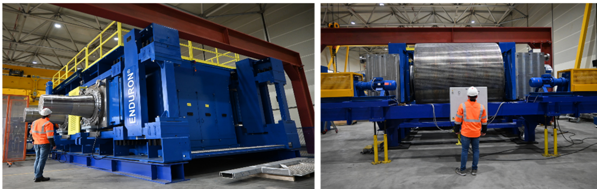
Figure 2—Enduron 2.6 Metre (m) Diameter x 2.6 m HPGR, Capable of Processing >6,000 tonnes per hour per Unit
