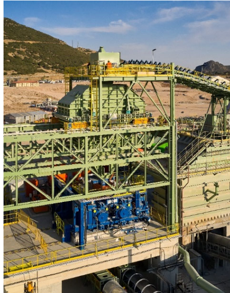
Figure 4—2.4 Metre-Diameter Enduron HPGR in PPR Circuit Configuration Feeding Gold Heap Leaching Pad
