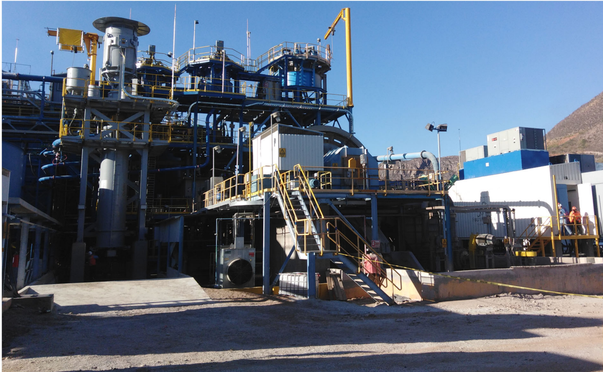
Figure 7—Ball Mill, Two-Stage Classification and VRM
