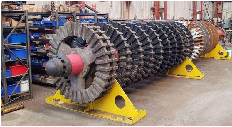
FIG 9 - Rotor assembly with flat rubber castellated rotors prior to despatch from MO workshop
