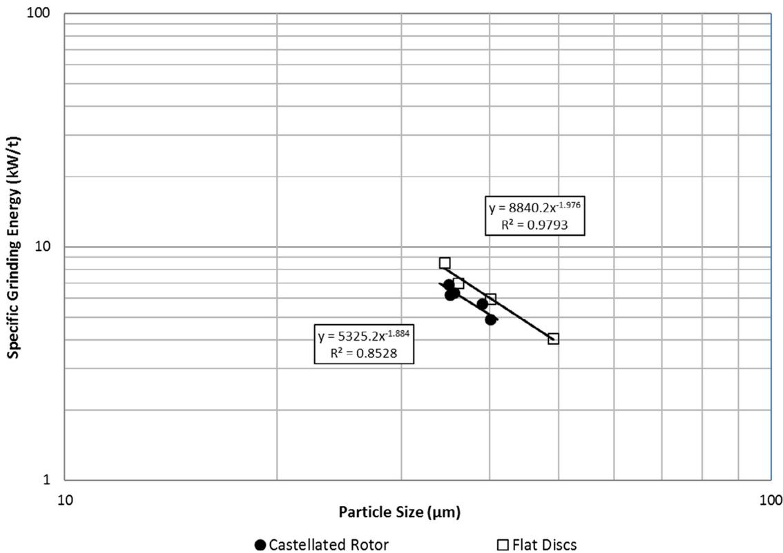
Fig. 9. Specific Grinding Energy (kWh/t) versus the particle size ( $P_{80}$ ,  $\mu\text{m}$ ) for Case A.
