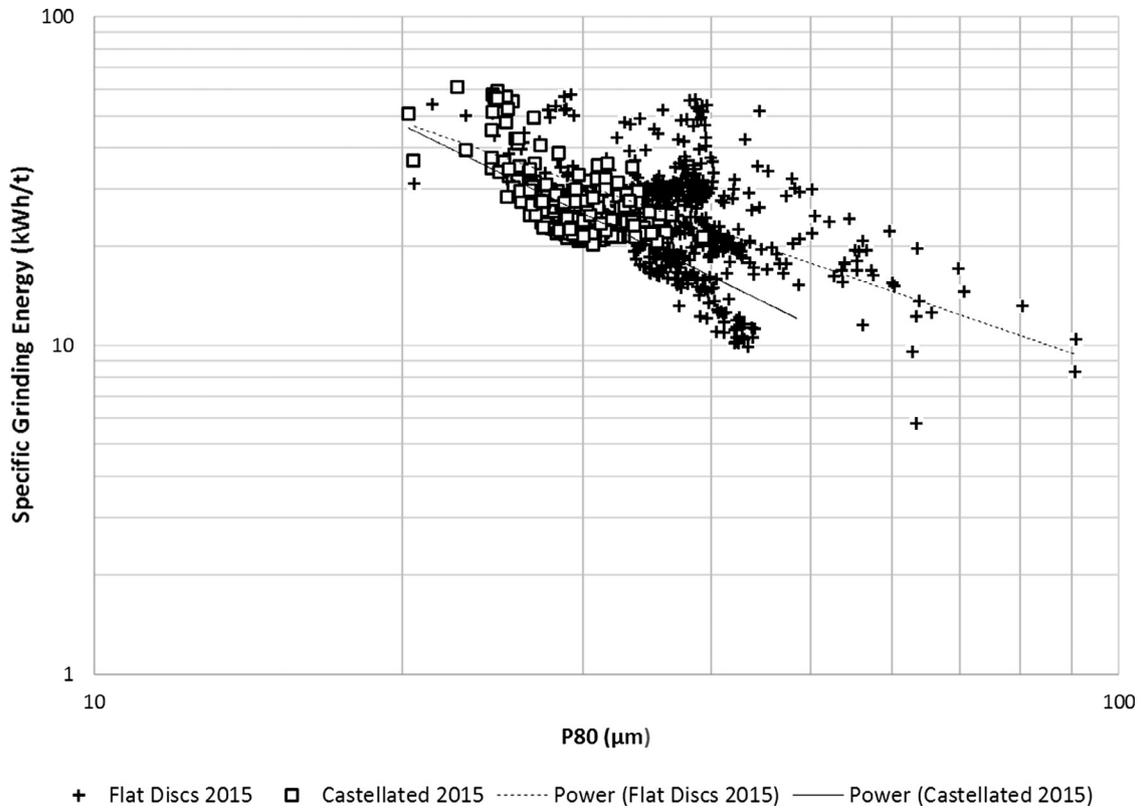
Fig. 5. Specific Grinding Energy (kWh/t) versus the particle size ( $P_{80}$ ,  $\mu\text{m}$ ) for Flat Discs versus Castellated Rotors in 2015.
