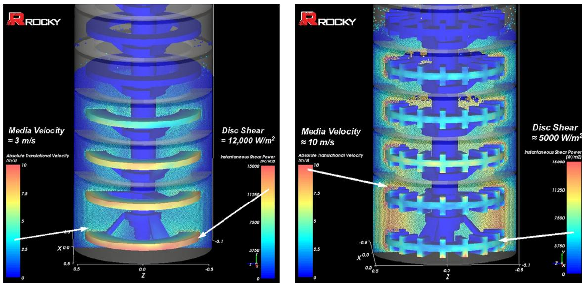
Fig. 1. Flat discs: energy goes into disc wear; castellated rotors: energy goes into grinding, from Heath et al. 2017.
