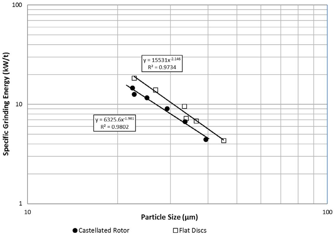
Fig. 10. Specific Grinding Energy (kWh/t) versus the particle size ( $P_{80}$ ,  $\mu\text{m}$ ) for Test Program B.
