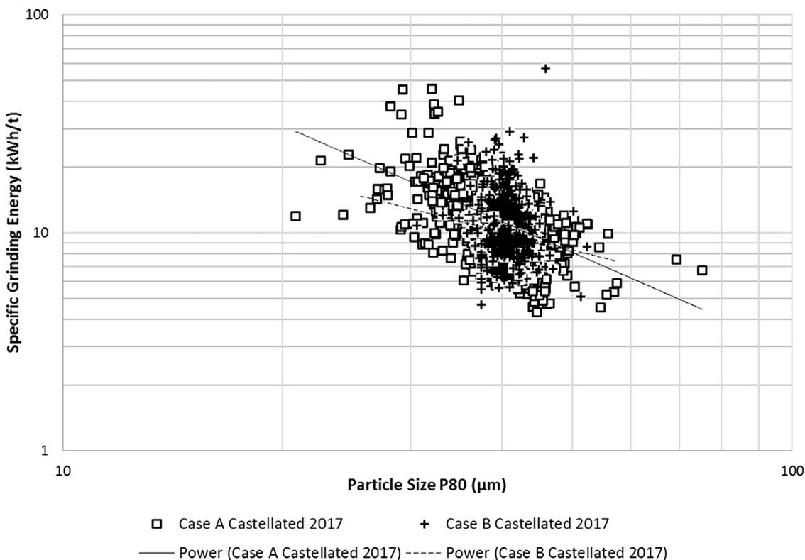
Fig. 7. Specific Grinding Energy (kWh/t) versus the particle size ( $P_{80}$ ,  $\mu\text{m}$ ) for Castellated Rotors Case A versus Castellated Rotors Case B in 2017.
