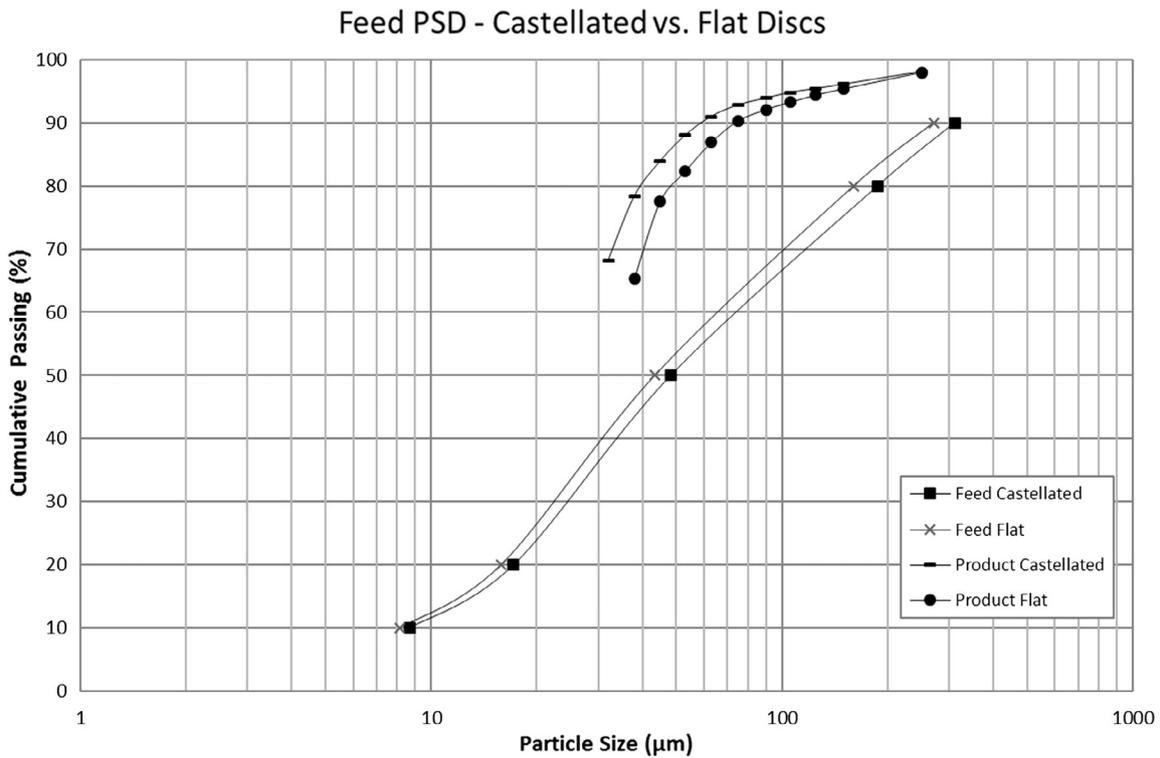
Fig. 11. Feed and product example of PSD for castellated and flat discs.
