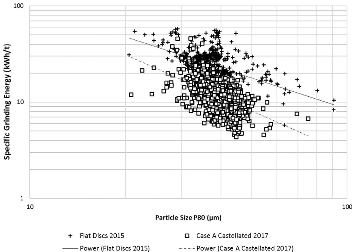
Fig. 6. Specific Grinding Energy (kWh/t) versus the particle size ( $P_{80}$ ,  $\mu\text{m}$ ) for Flat Discs 2015 versus Castellated Rotors Case A in 2017.
