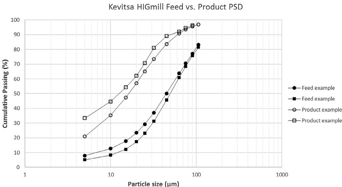
Fig. 8. Example of feed and product particle size distribution variation for Kevitsa HIGmill.
