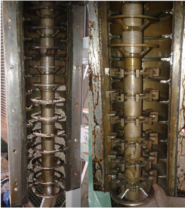
Fig. 3. Thin Flat Discs (left) and Castellated Rotors (right).
