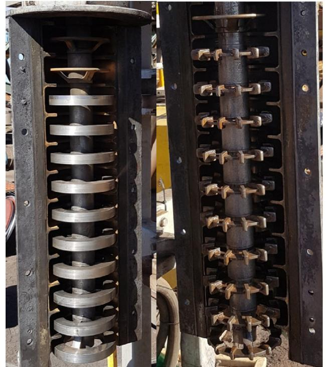
Fig. 4. Fat Flat Discs (left) and Castellated Rotors (right).
