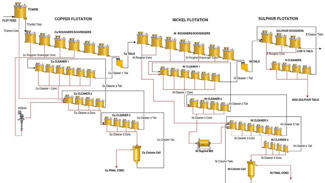
Fig. 2. Kevitsa flotation flowsheet (Lehto et al., 2016).
