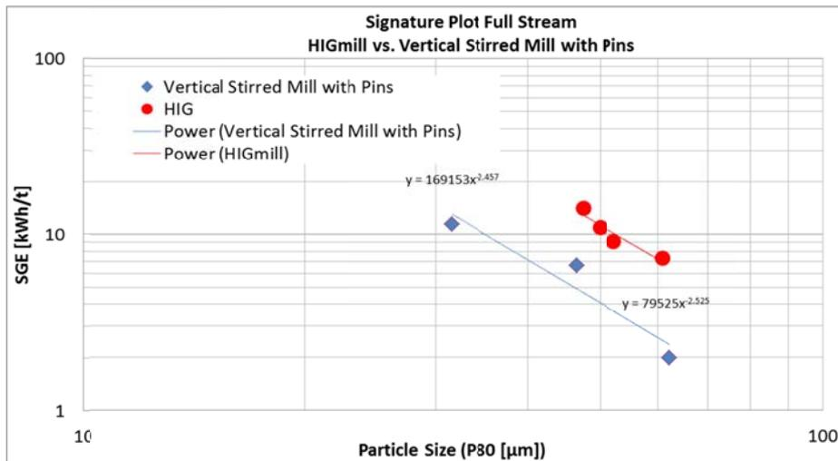
Figure 17. Signature plot full feed stream
