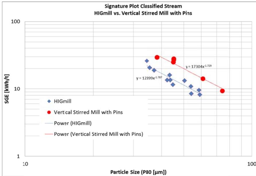
Figure 16. Signature plot classified feed stream
