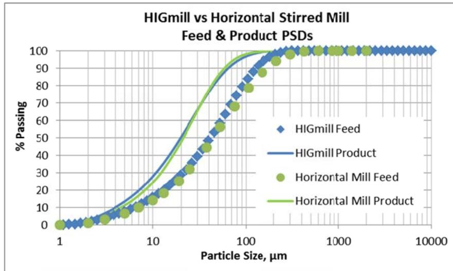
**Figure 14.** PSDs of the feed and product of both mills
