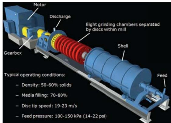
**Figure 6.** Horizontal stirred mill with flat grinding discs (H. de Waal et al., 2013)
