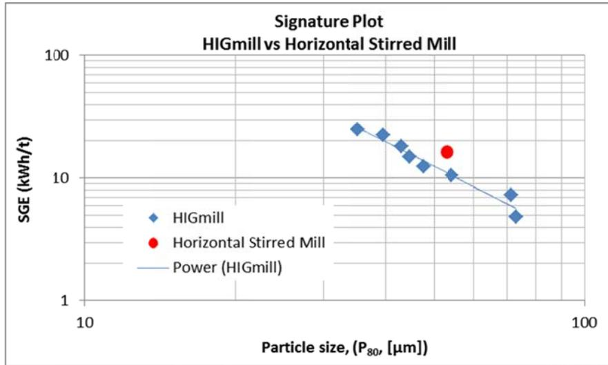
**Figure 15.** Signature plot of the HIG mill vs Horizontal Stirred mill
