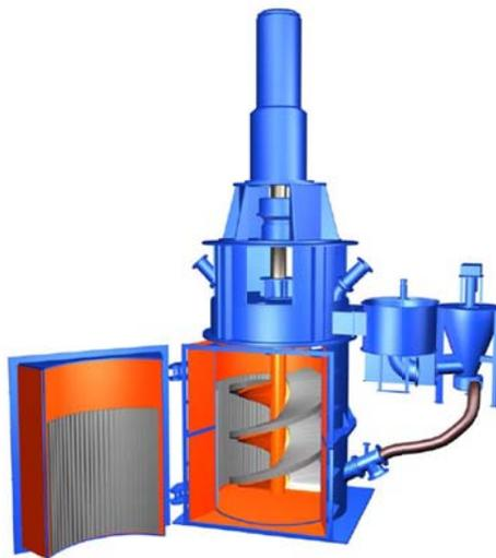
**Figure 3.** Vertical tower mill with helical agitator (J. Allen, 2009)
