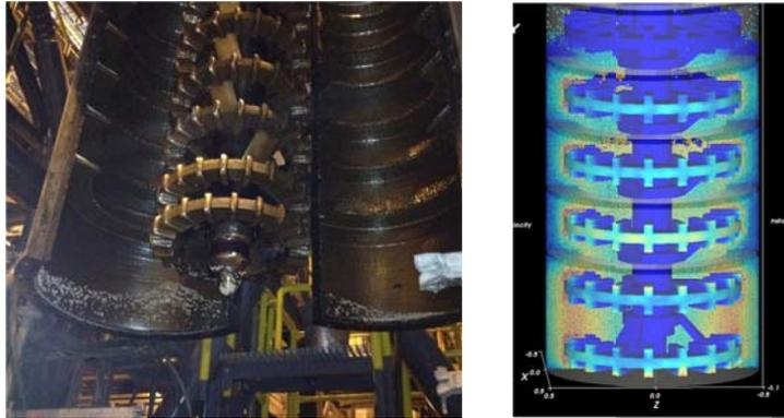
**Figure 2.** Special shaped vane rotors in the Outotec HiGmill™
