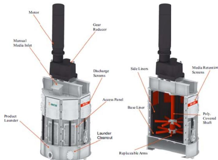
**Figure 5.** Vertical stirred mill with pins (C. Ntsele et al., 2012)
