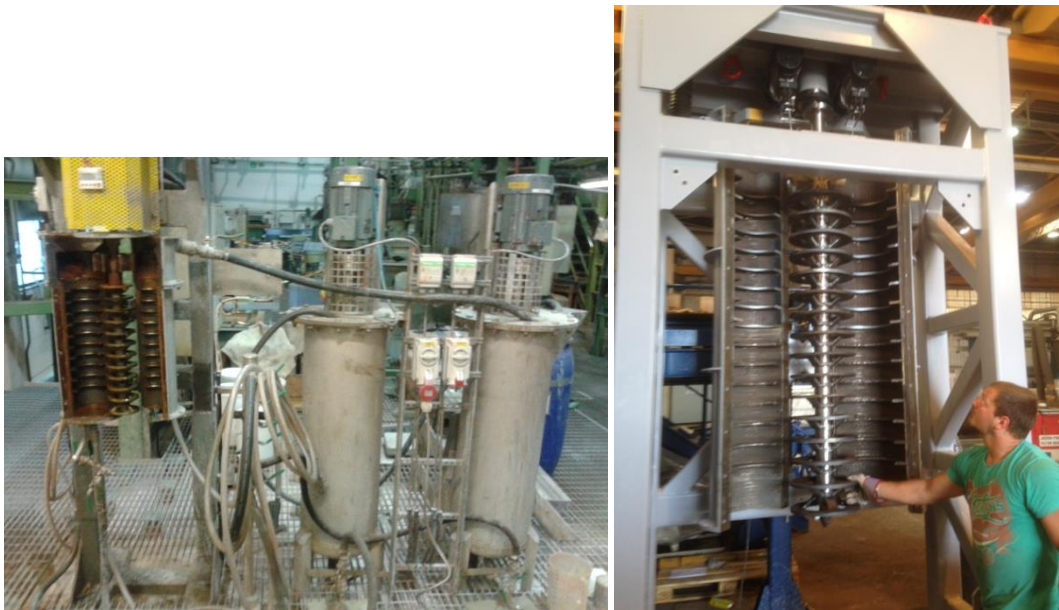
Figure 11. Outotec HiG 5 test set up (left)(Junnola 2013), and HiG 75_200 (right) (KMF 2014)
