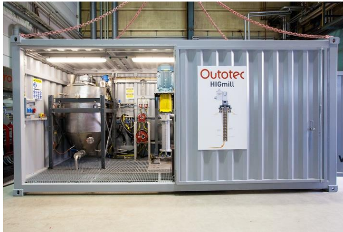
Figure 10. HiG25 container unit. (Outotec, 2013).
