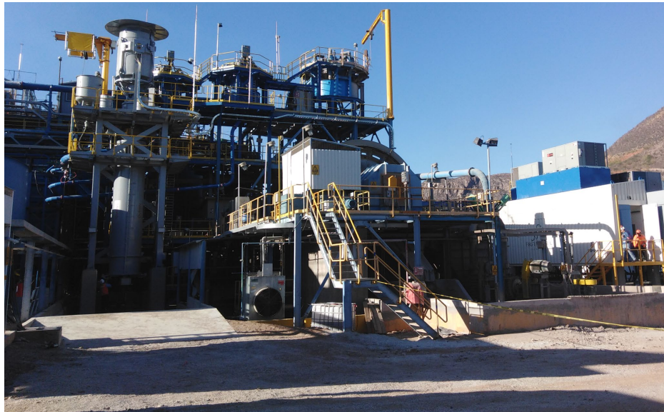
Figure 10 – HIGmill and the two-stage classification system
