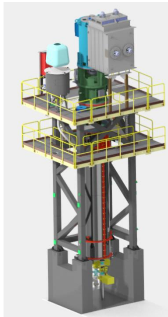
Schematic impression of a VRM mill
