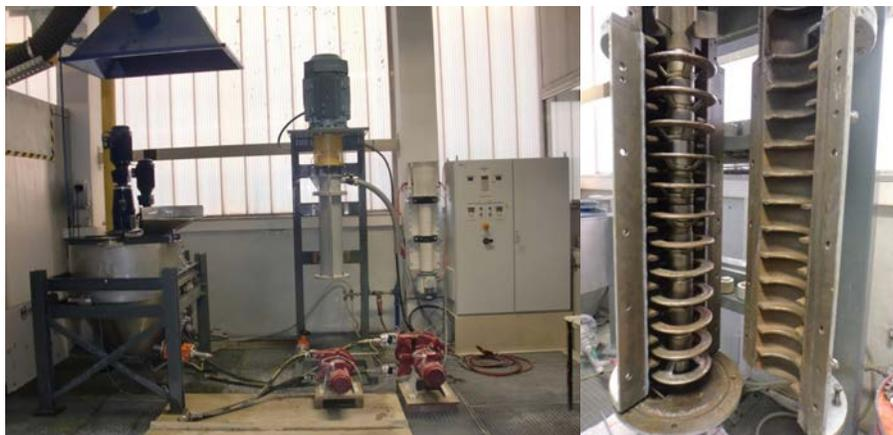
Figure 3 – HIG25 laboratory test mill with auxiliaries and mill internals
