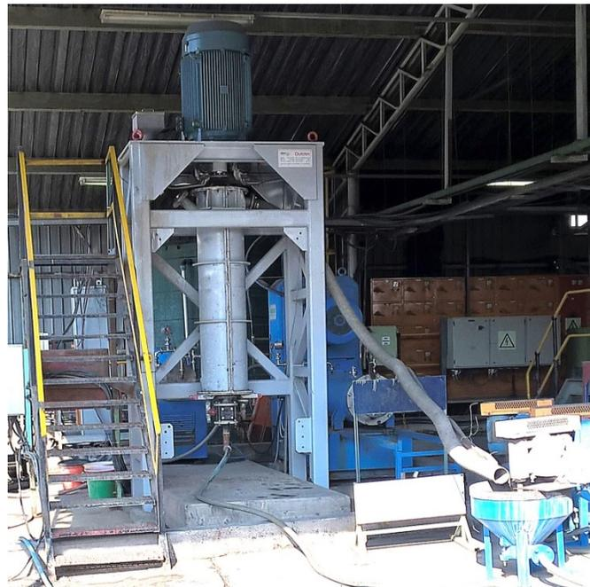
Figure 6 - The HIG 200/75 installed at AAP's DML Pilot Plant
